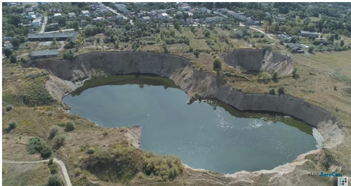
Figure 4.17: Anthropogenic salt karsts formed by salt mining and subsequent water intrusion Source: https://ua-reporter.com/
